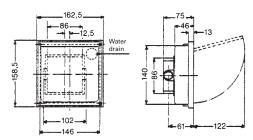
If unit is floor mounted, the knockout in the base should be used as an outflow in the event of water seeping in.
